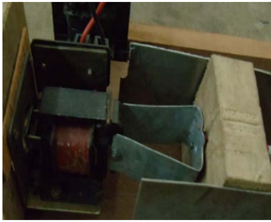
Figure 6: The brake coil is energized
