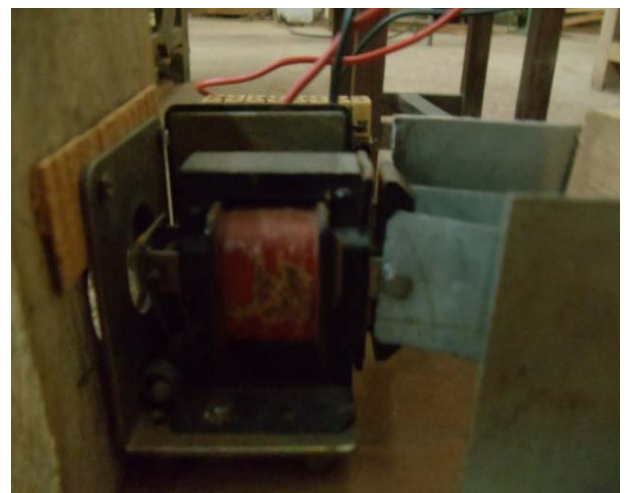
Figure 2: Brake coil
